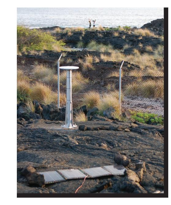
immediately following the October 15, 2006 M6.7 Kiholo Bay USGS/Hawaii Volcano Observatory. This and four other stations will be used to determine the post-seismic deformation field
