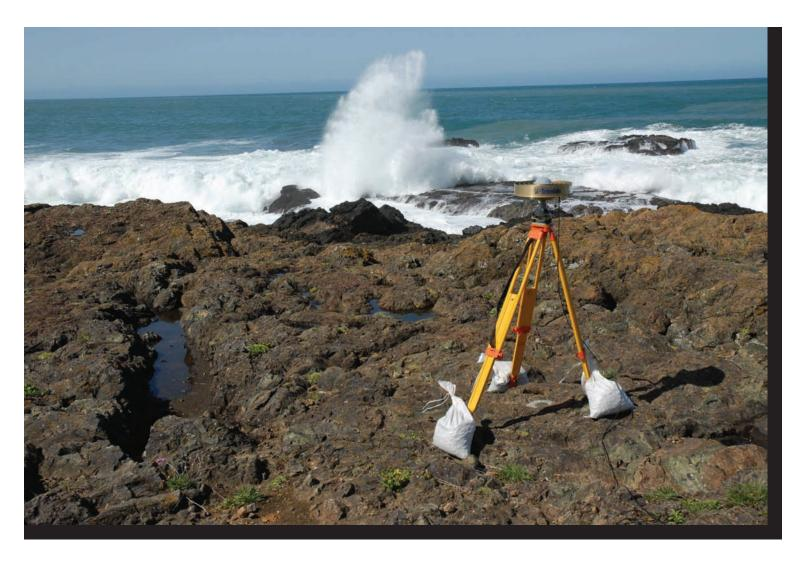
San Andreas Fault system airborne LiDAR survey. Topcon GB-1000 receivers recorded 1 Hz data collected by tripod-mounted choke rings over existing first-order benchmarks. Data was used to determine the locations of the aircraft and scanner to improve the resolution of the LiDAR images. The stations were manned by UNAVCO personnel and by USGS volunteers while missions were being flown.
