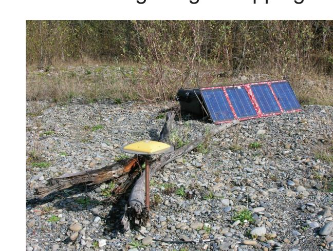
Above: Campaign GPS station on the Olympic Peninsula, WA. Low profile antenna mounts were used to reduce the amount of equipment to be transported into remote areas. 32 watt solar panels provide the power necessary to run the Topcon GB-1000 GPS receiver for the duration of the experiment. (Univ.'s of WA and AZ)
