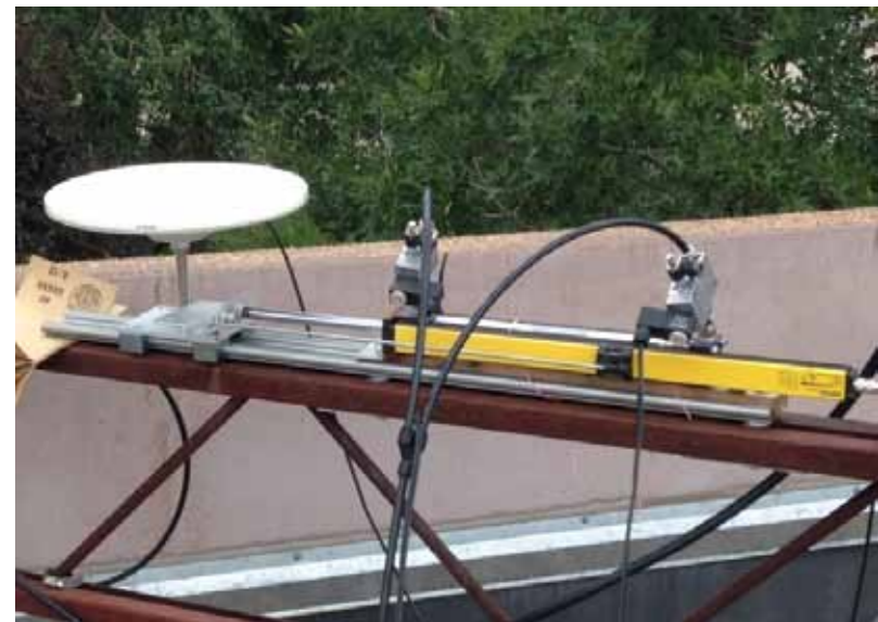
Left: A low-cost antenna actuator utilizing a pneumatic cylinder for controlled 1-d antenna motion. The maximum displacement of the staged is limited to ~300mm. Antenna displacement is measured independently from GPS using a Turck linear position sensor. The system is controlled by a Raspberry Pi and a simple micro controller. The precise displacement measurements are logged using a Kinemetrics Basalt Rock data logger.
