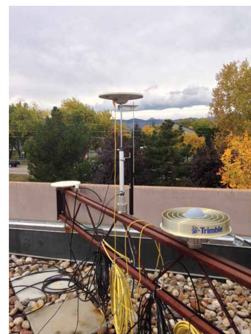
Pneumatic cylinder with 300 mm maximum displacement showing Trimble Zephyr antenna and linear position sensor attached. The antenna cable lead into the building and connects to a splitter where multiple receivers can track simultaneously.
