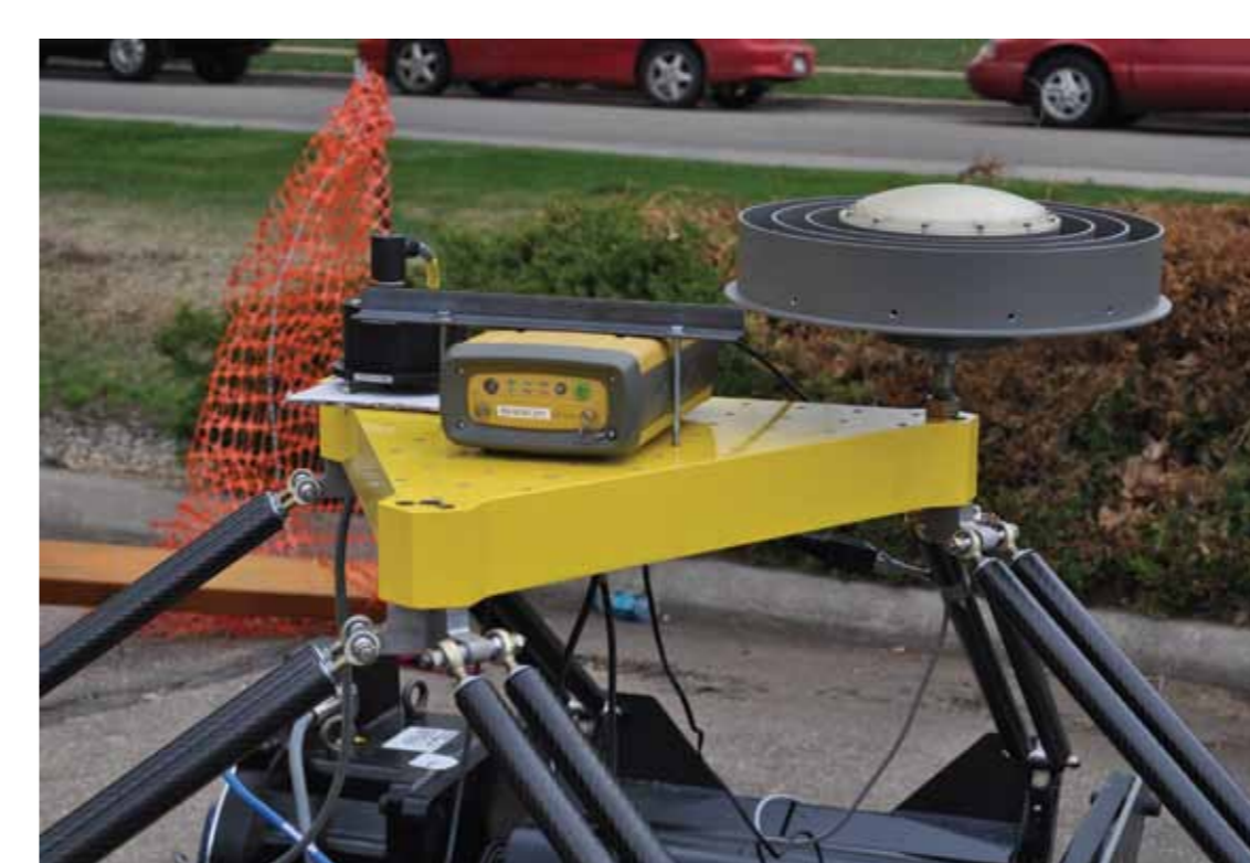
A close up of the shake table apparatus. Each receiver was fixed to the table using angle iron anchored with 1/4" bolts. The table design consisted of three very large DC servos connected to a triangular table with carbon rods. The table's capacity was limited to 200 lbs. The table's maximum acceleration was limited to 8g.
