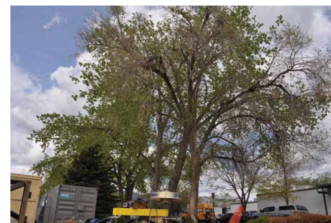
The testing locality provided a challenging environment for GNSS tracking. (Above) A photo of the test site looking to the NW. A large tree obstructs the sky view.
