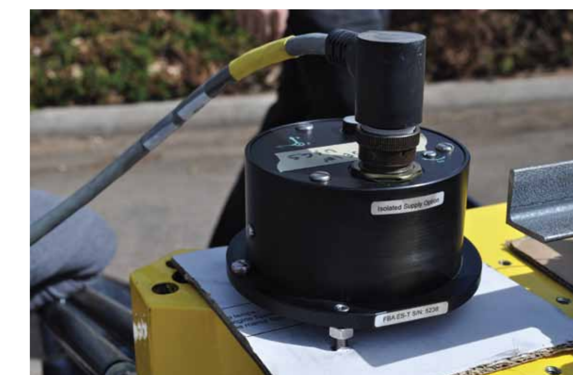
A Kinemetrics EpiSensor ES-T was also affixed to the table allowing 100 sps measurements of acceleration in the X, Y and Z components. The measurement range of the ES-T was limited to \pm 4g . Clipping occurred during the experiment when accelerations exceeded 4g.
