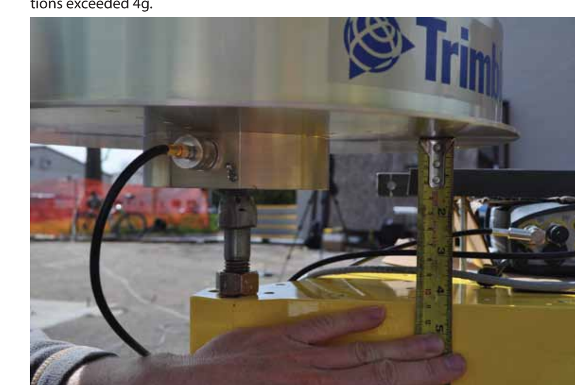
Each test antenna was fixed to the NE corner of the shake table using a 3/4" to 5/8" threaded stud. Locknuts were used to prevent the antenna from loosening during the test. The antenna ground plane was ~4" above the surface of the table.
