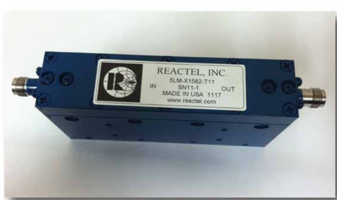
Above: Gain vs. frequency for a Trimble GPS Choke Ring antenna LNA compared with a Trimble GNSS Choke Ring LNA. The bandwidth of the newer GNSS choke ring has been increased to improve the tracking of GNSS signals. Right: A custom cavity-type notch filter designed to mitigate the interference caused by Iridium communication transmissions.
