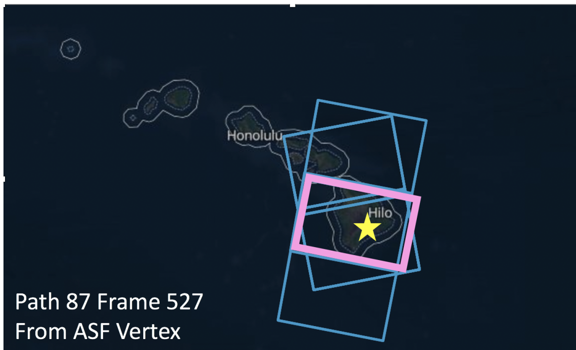
Figure 6: SAR footprint of Path 87 Frame 527 coverage over Hawaii that was used for processing. Data was downloaded using the ASF Vertex portal.
