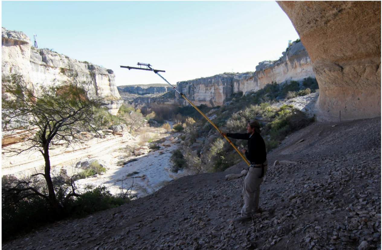
Figure 2. Pole aerial photography (PAP) platform. This example is from an archaeological site in Texas; the person is photographing the talus slope. Note the angle required to photograph given the camera cannot be oriented straight down. Source:
