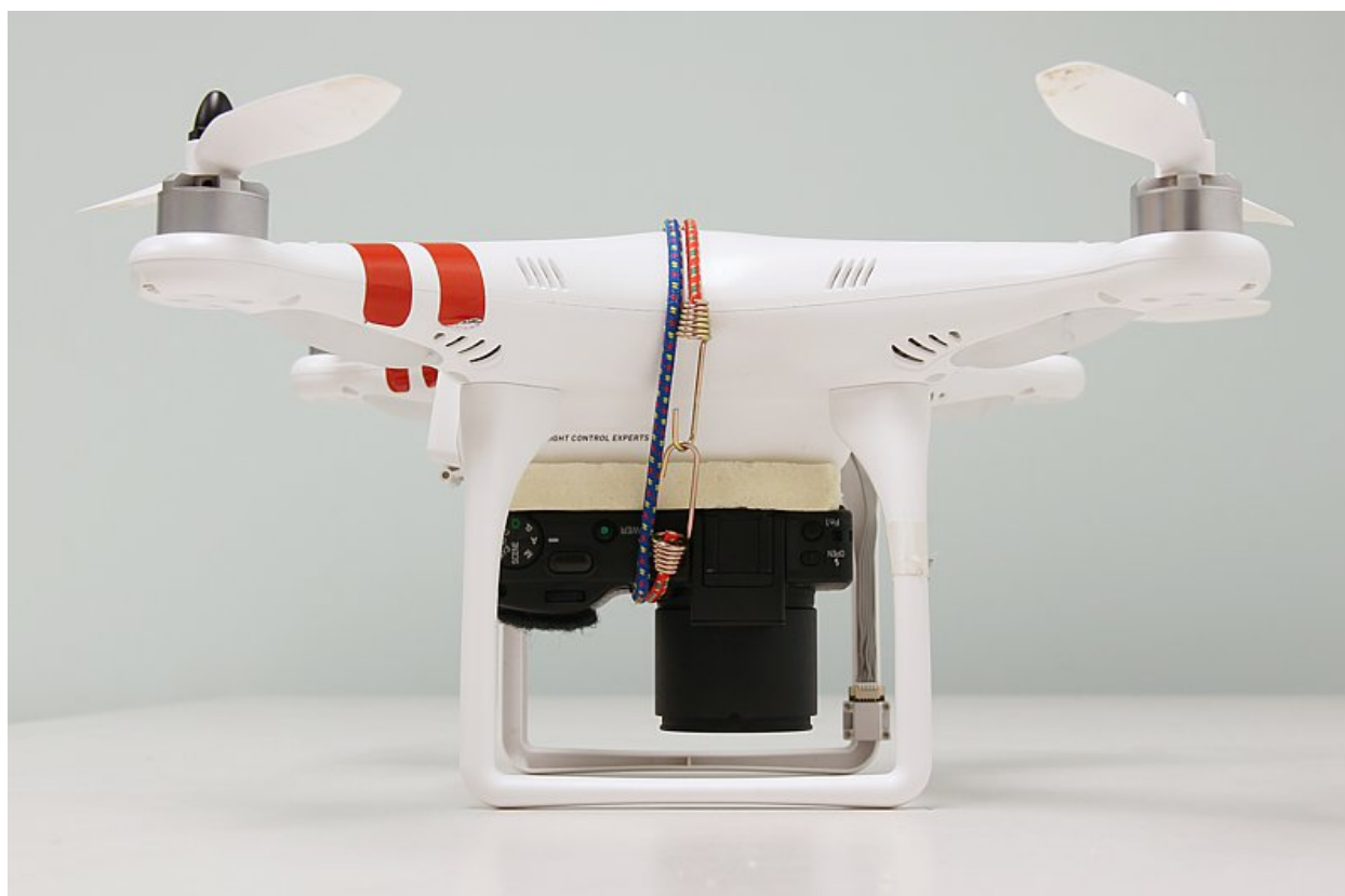
Figure 6. Examples of pre-made and built UAV camera mounts. The top image is of a typical camera mount available to purchase in most hobby shops for UAVs. The example below is a camera attached to a quadcopter using bungee cords and a piece of foam padding to reduce the vibration transmitted to the camera. Sources: Turner et al. (2012), Remote Sensing, and http://www.paulillsley.com/airphoto/systems/Phantom/ (accessed July 1, 2015)
